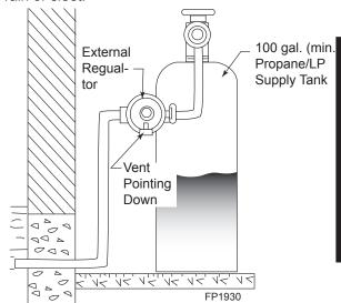
Figure 12 - External Regulator with Vent Pointing Down (Propane/LP Only) Use only new black iron or steel pipe. Internally tinned copper or copper tubing can be used per National Fuel Gas Code, Section 2.6.3, providing gas meets hydrogen sulfide limits, and where permitted by local codes. Gas piping system must be sized to provide minimum inlet pressure (listed on data plate) at the maximum flow rate (BTU/hr). Undue pressure loss will occur if the pipe is too small.
